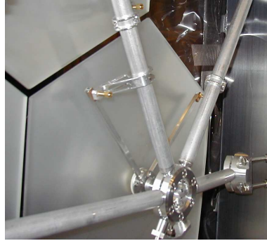
Figure 5.34: Mirror wall rear face, detailed view: the mechanical arrangement for the angular adjustment of an individual mirror element is visible.
