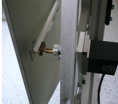
Figure 5.36: Laboratory setup, the mirror rear side: the piezo actuator replaces one of the micrometric screws.
